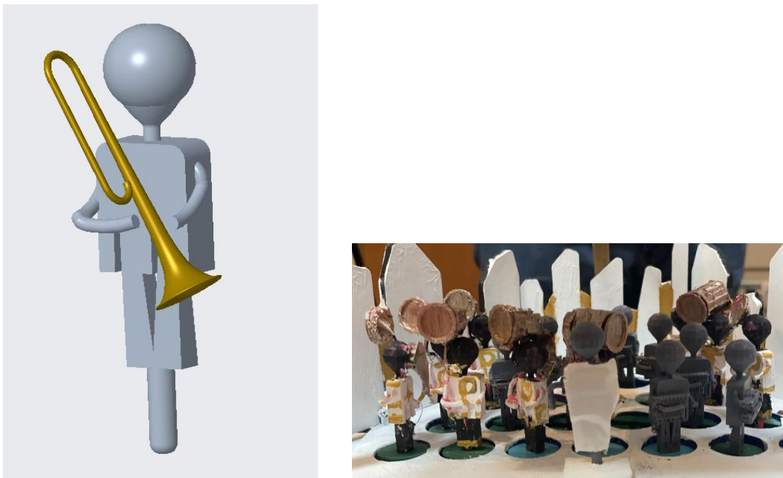
Figure 3.4.1: CAD model of a trumpet figurine (left) and the prototype result (right)
